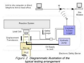
A separate gauge is used to monitor the displacement of the pile head with respect to the underside of the reaction beam; this allows a secondary measurement of pile head movement and load applied as well as necessary verification of the integrity and reliable operation of the reaction system.
